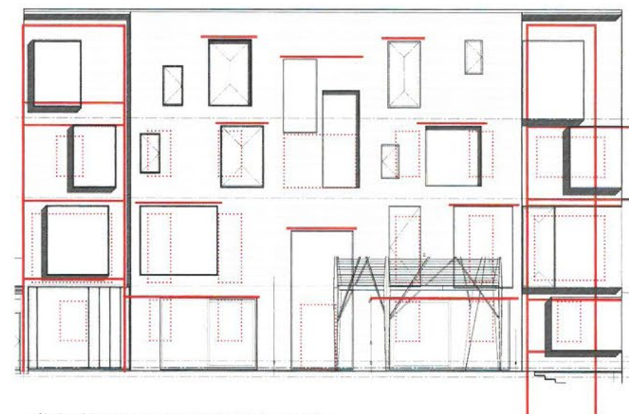
■ Study of the new apertures on the interior elevation superimposed on pre-existing openings
